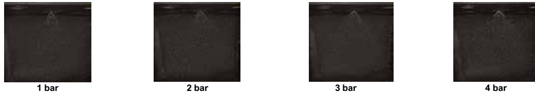
Fig.3 Spray shape at different P_{inj} with L_o/D_o=0.22 , W \times H=1.5 \times 1.5 \text{ mm}^2 , \theta = 90^\circ and L_s/D_s = 0.93 for ESPSA of 30 kV after image processing.
