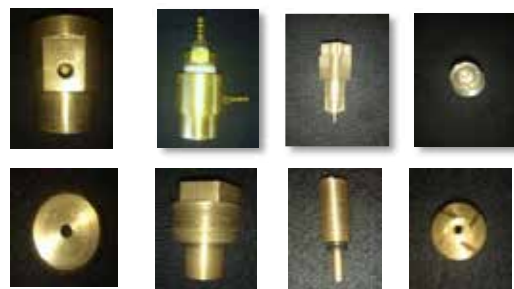
Fig. 2. Components and assembly of the conventional PSA and electrostatic pressure swirl atomizer (ESPSA).
