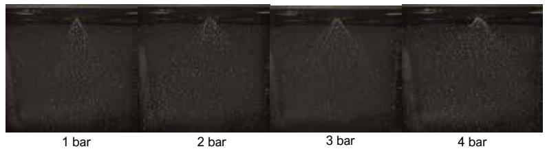
Fig.1. Effect of Injection Pressure P_{inj} on the EPSA at 30 Kv with fixed geometry
